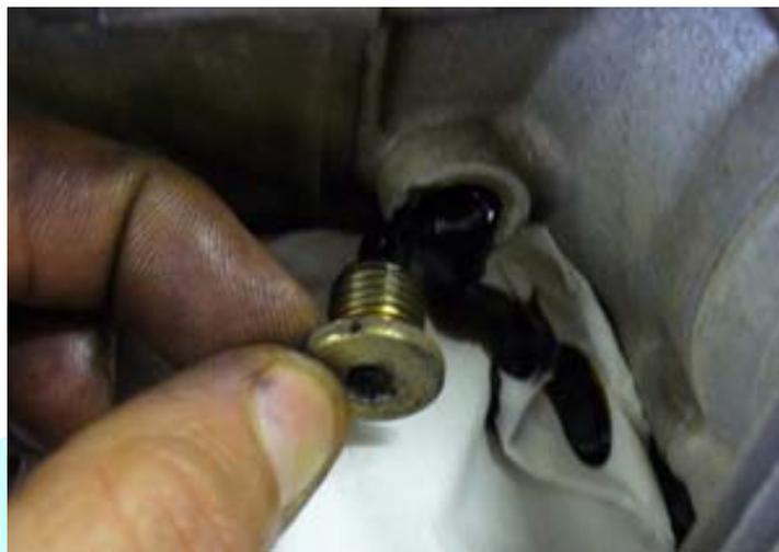
Figure 28: Oil behind magnetic plug
