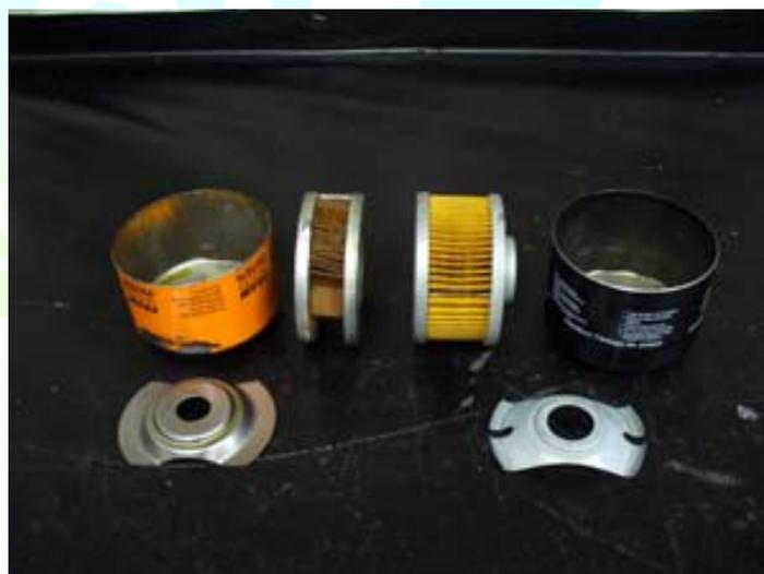
Figure 26: Genuine filter and pattern one. Pattern filter is on left with much smaller filter area.
