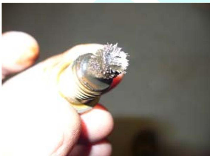
Figure 29: furred magnetic plug before cleaning
