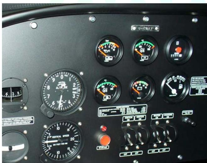
Figure 3: Instrument marking kit fitted to a Eurostar
