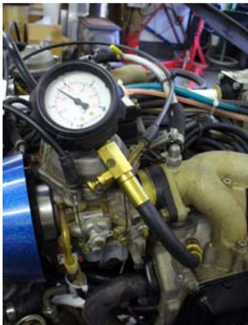
Figure 50: Conventional automotive style compression tester
