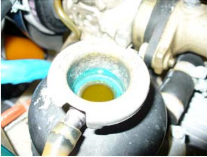
Figure 16: Corroded expansion tank
