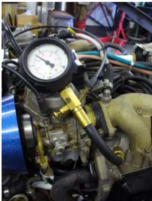
Figure 50: Conventional automotive style compression tester
