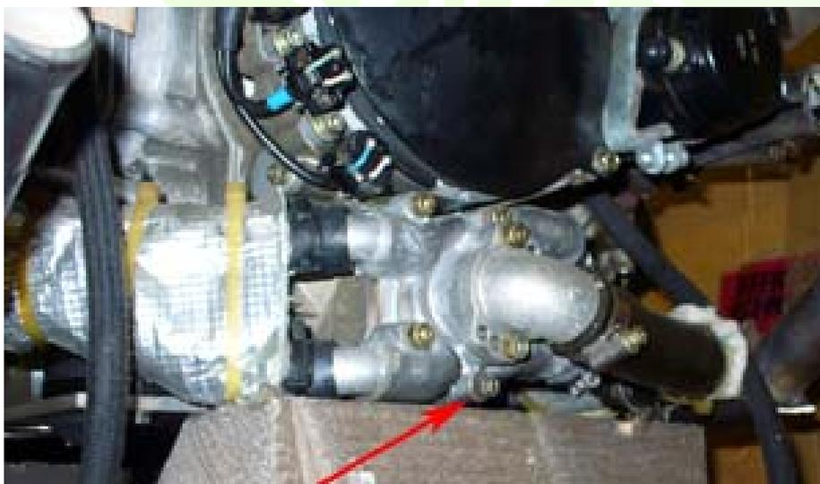
Figure 52: Water drain screw on water pump
