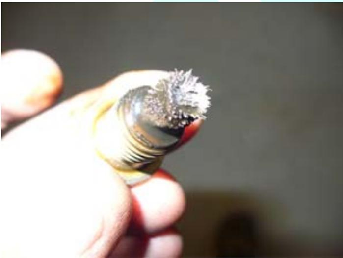
Figure 29: furred magnetic plug before cleaning
