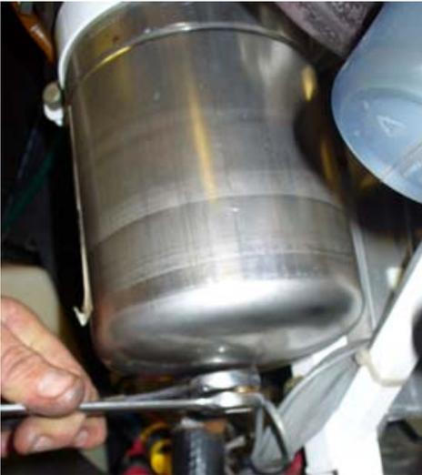
Figure 18: Undoing oil tank drain bung
