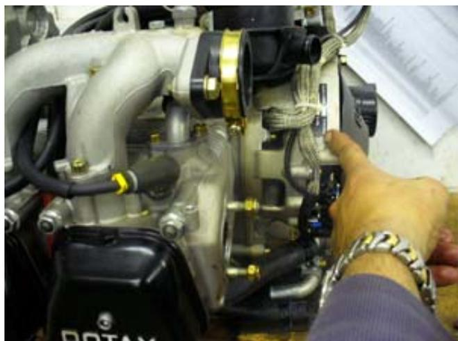
Figure 5: Position of engine serial number
