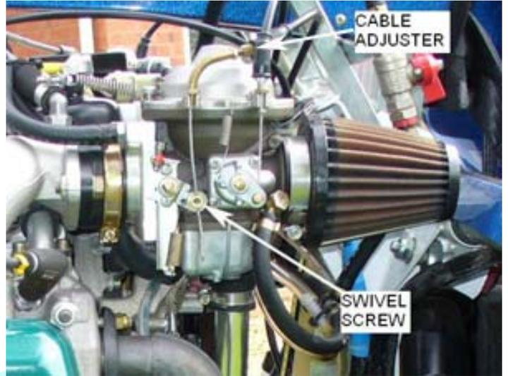
Figure 40b: Sprung closed throttle system
