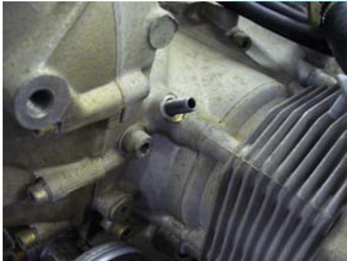
Figure 48: Crankshaft locking pin location
