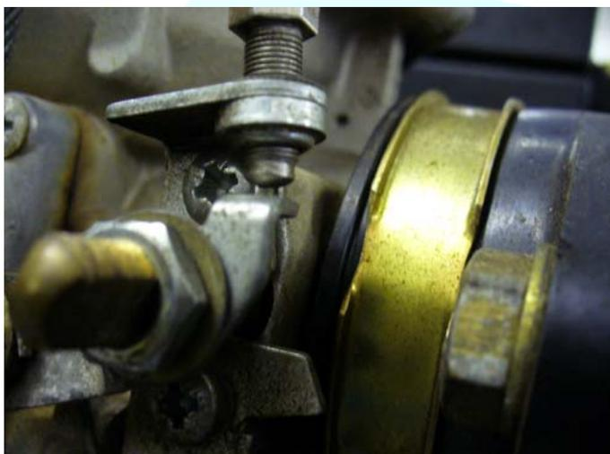
Figure 42a: Throttle idle screw clear of lever.
