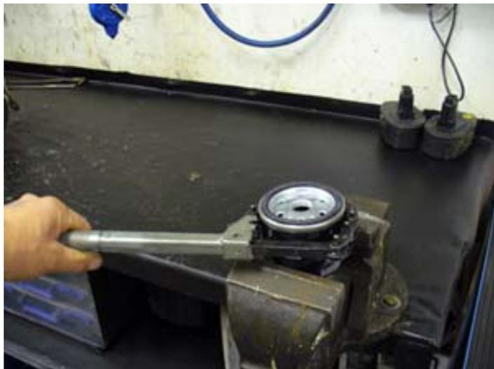
Figure 23: Cutting open the filter
