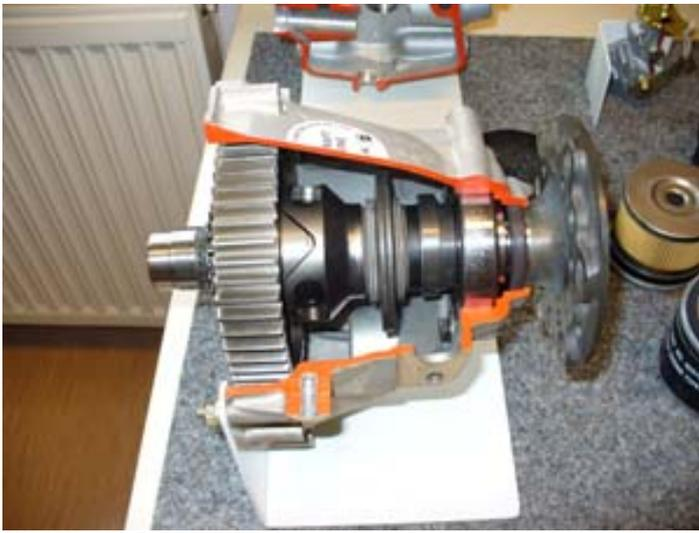
Figure 47: Gearbox without slipper clutch
