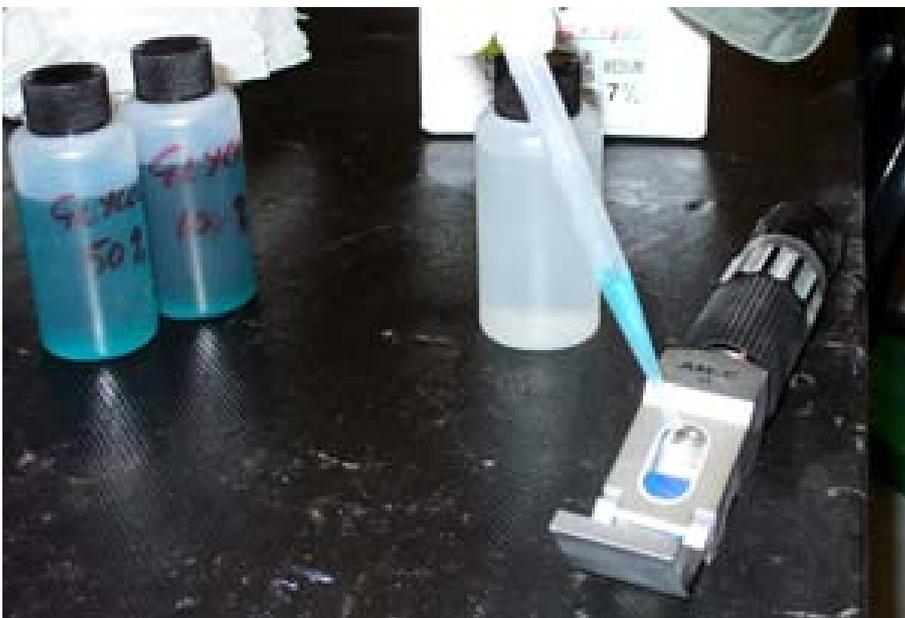
Figure 14: Using refractometer to check glycol ratio
