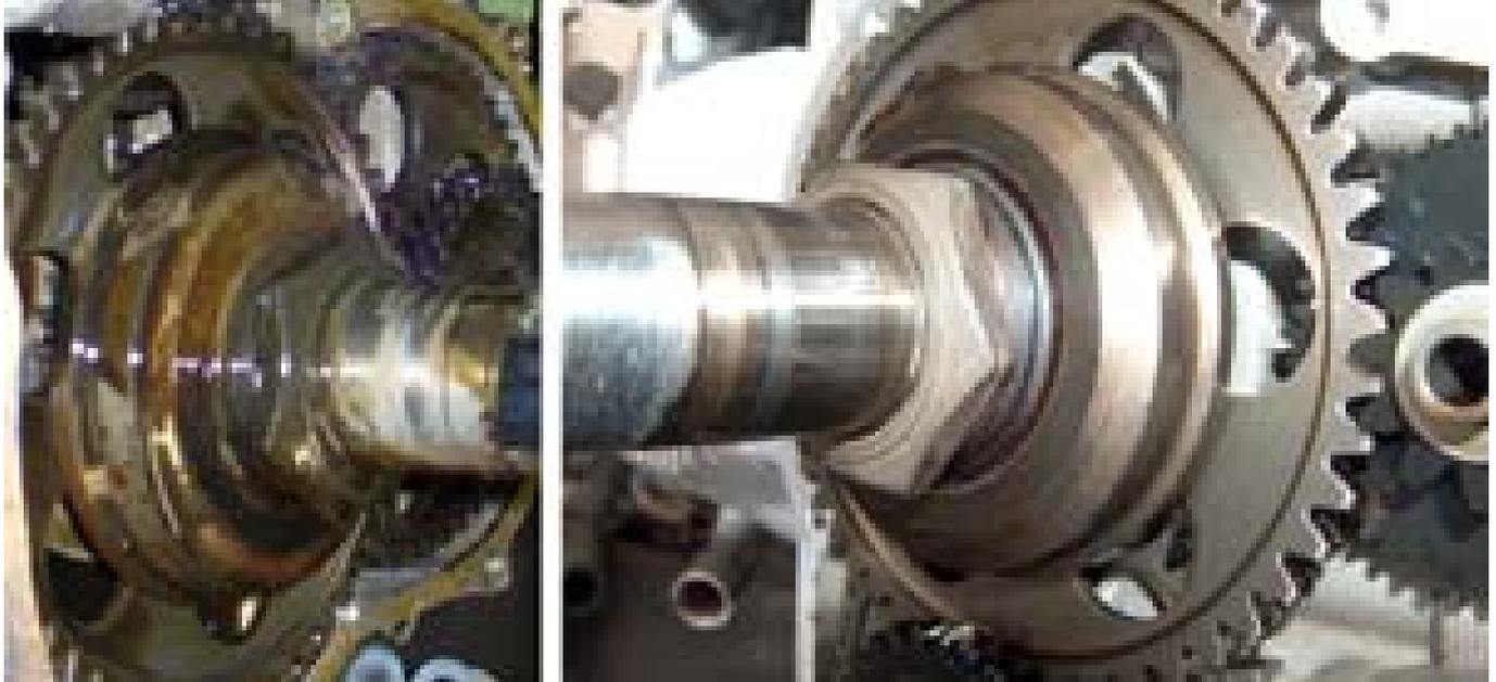
Figure 7: Sprag clutch in an engine run on Avgas (left) and the same component in an engine run on Unleaded Mogas
