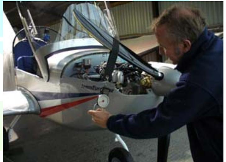
Figure 49: measuring friction torque at ½ m on the prop
