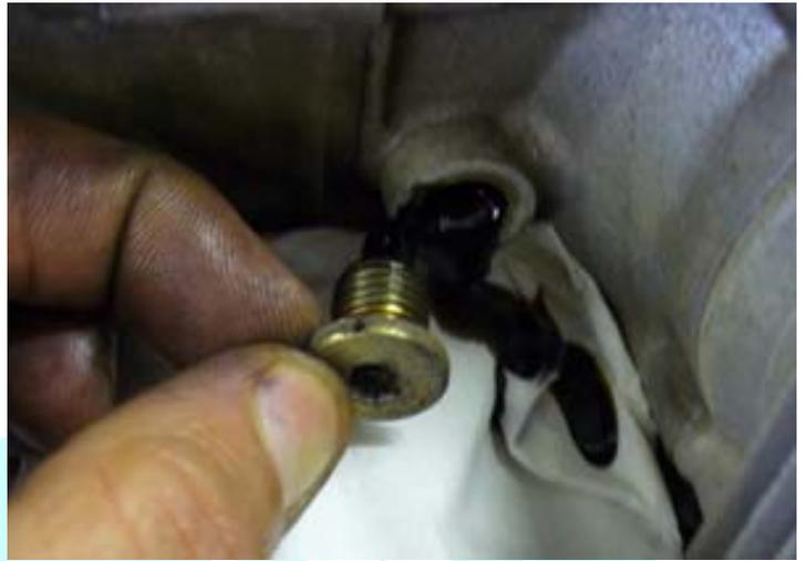
Figure 28: Oil behind magnetic plug
