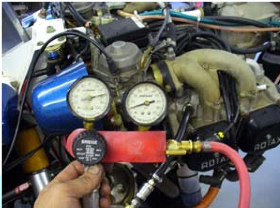
Figure 51: Leak down (differential) compression tester
