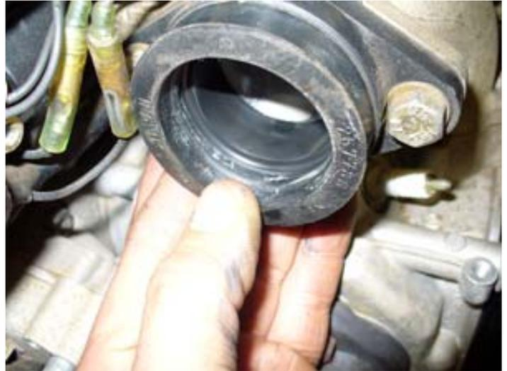
Figure 39: Checking carb rubber flange for cracks
