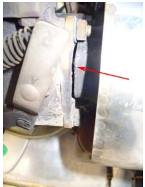
Figure 15: Crack in 914 exhaust pipe.
