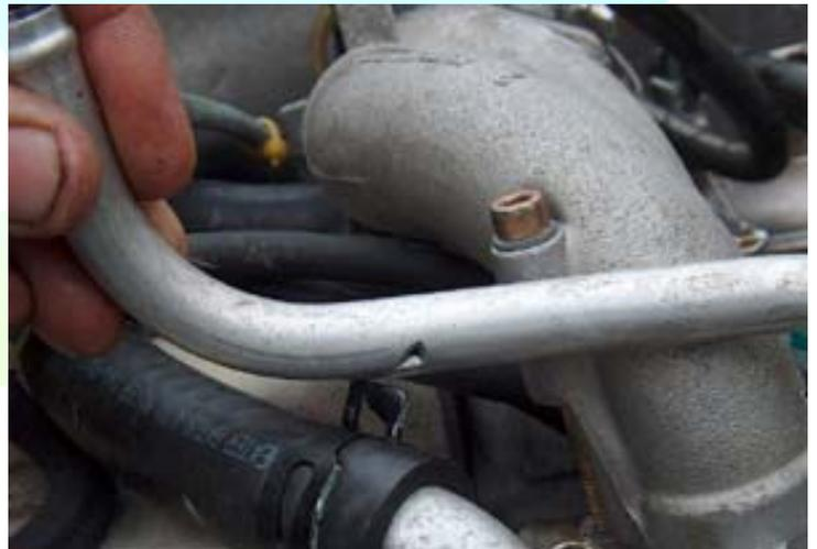
Figure 13: Oil tube worn through on hose clamp
