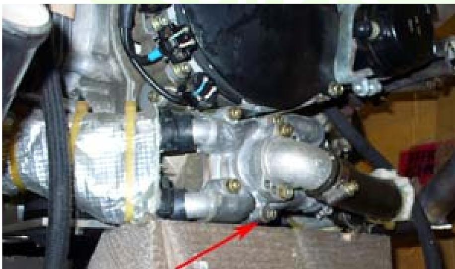
Figure 52: Water drain screw on water pump
