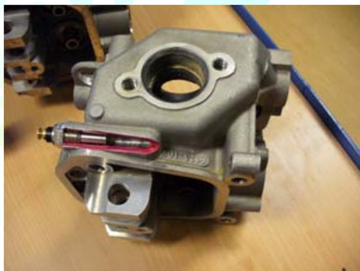
Figure 4: Cylinder head temp probe on cylinders 2/4 (not water temp)
