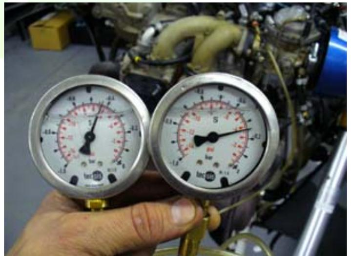
Figure 42: Pneumatic carb balancers
