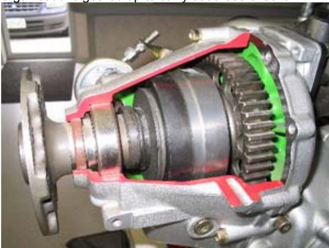
Figure 44: Gearbox with slipper clutch
