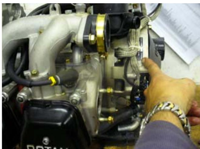
Figure 5: Position of engine serial number
