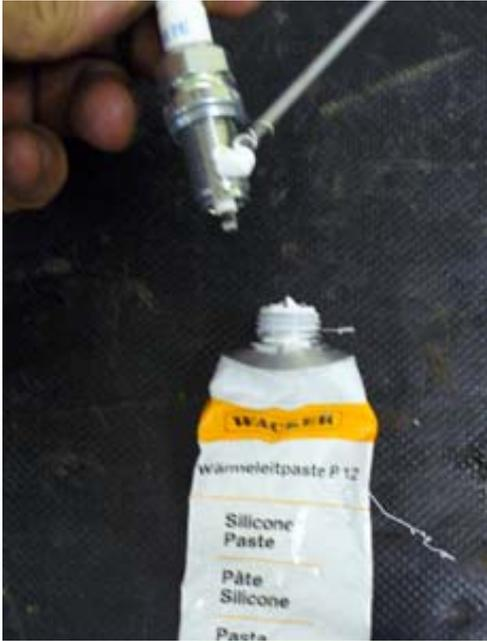
Figure 32: Applying heat sink paste
