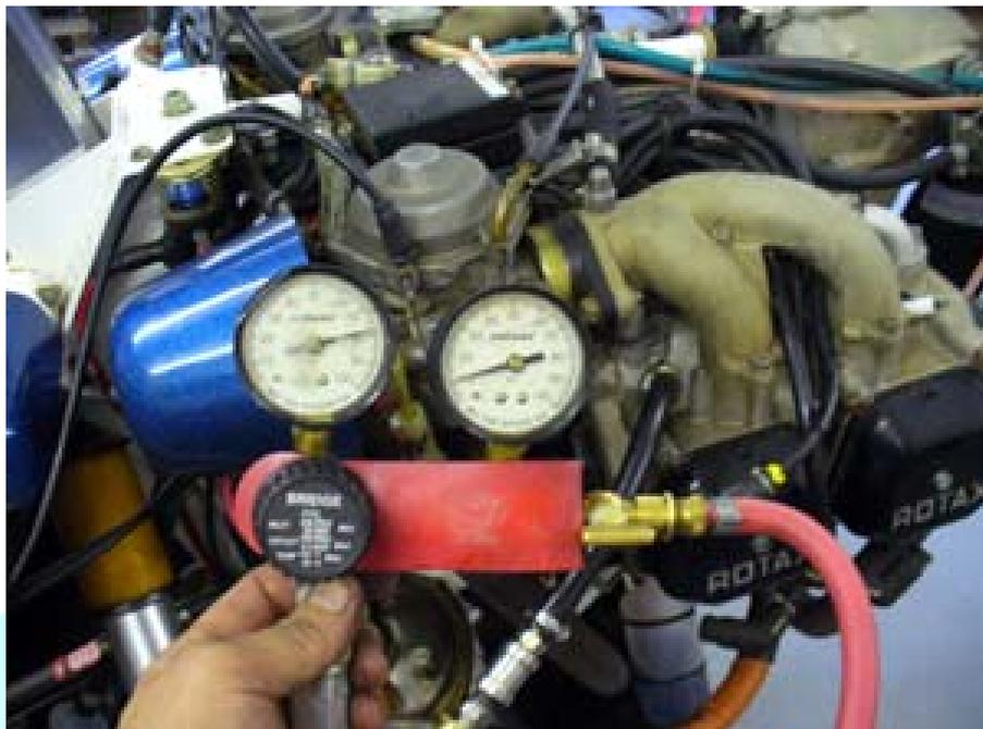
Figure 51: Leak down (differential) compression tester
