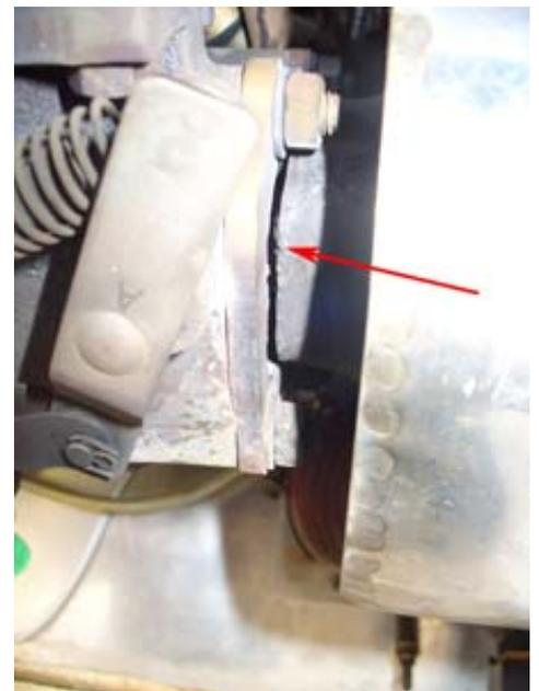
Figure 15: Crack in 914 exhaust pipe.
