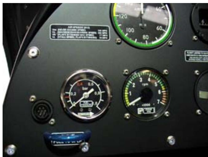
Figure 11: Fuel pressure gauge fitted
