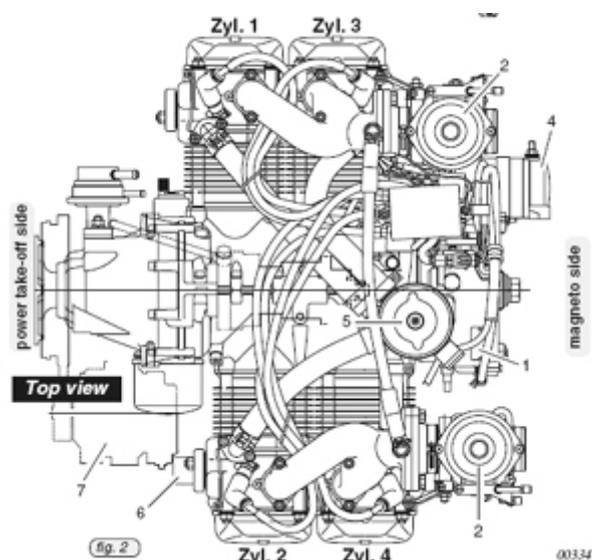
Figure 6: Drawing of cylinder orientation
