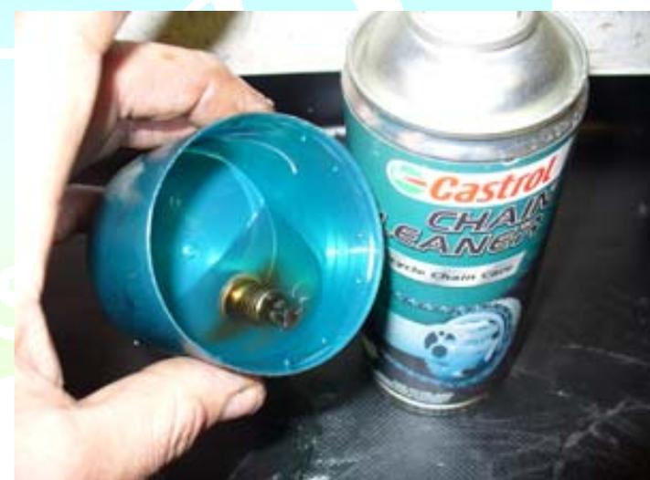
Figure 30: Cleaning magnetic plug
