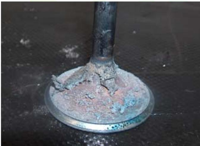
Figure 8: Valve after 1000 hours Avgas use
