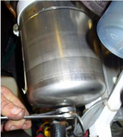
Figure 18: Undoing oil tank drain bung
