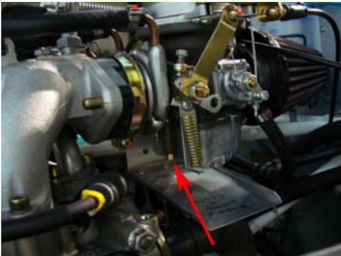
Figure 41: Photo 37 of idle mixture screw (hex).
