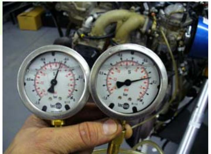
Figure 42: Pneumatic carb balancers
