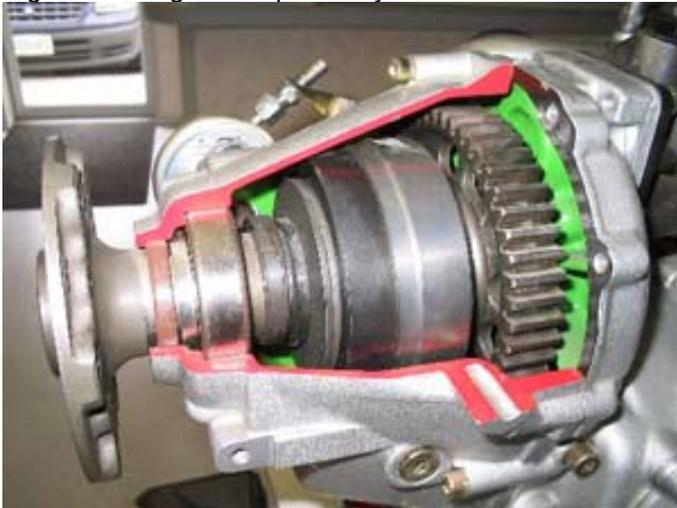
Figure 44: Gearbox with slipper clutch
