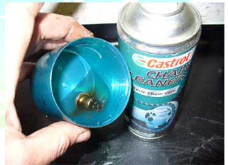
Figure 30: Cleaning magnetic plug
