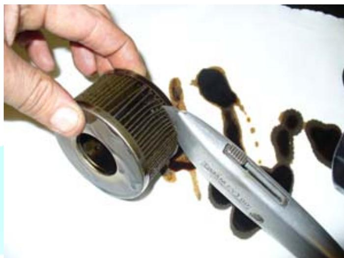
Figure 24: Removing the filter paper.
