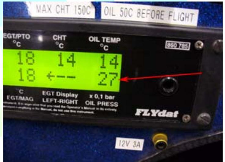
Figure 21: Flydat showing 2.7 bar oil pressure
