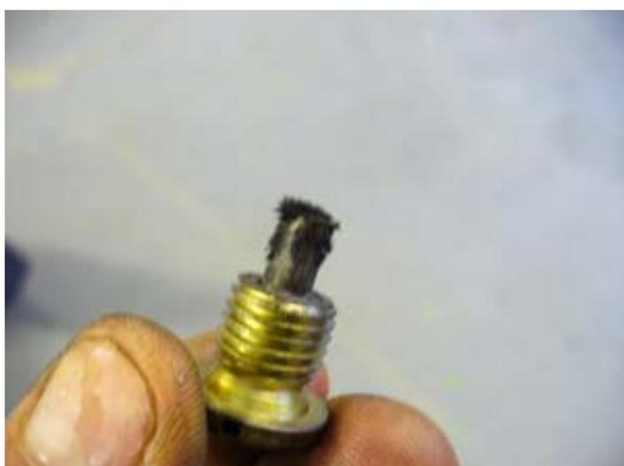
Figure 31: Plug after cleaning in carb cleaner
