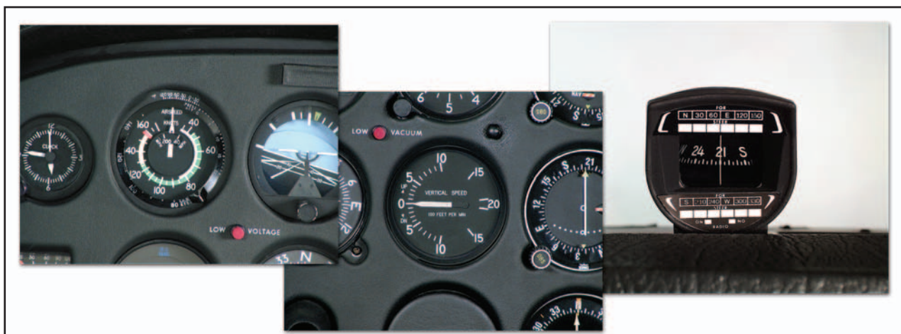
Figure 2-5. Airspeed indicator, VSI, and magnetic compass.
