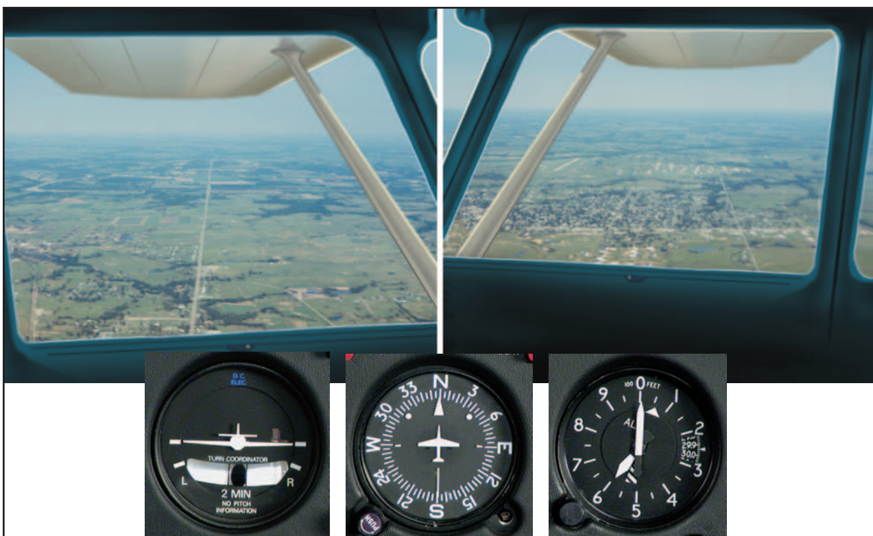
Figure 3-4. Wingtip reference for straight-and-level flight.
